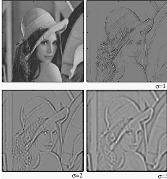
Figure 6.17 – Gaussian derivative for \sigma_1 = \{1, 2, 3\} and \sigma_2 = 1.4\sigma_1
