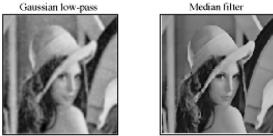
Figure H6.9 – Suppression of the snow by gaussian-smoothing filtering (image on the left) and by median filtering (image on the right)
